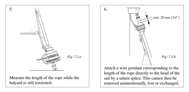
7. All the boat's foresails must be adjusted to the correct luff length.
