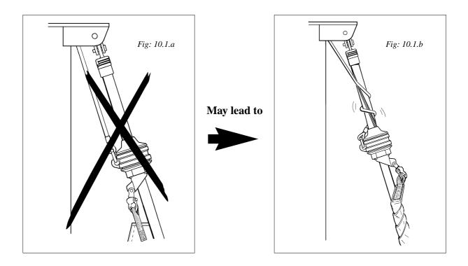
When sailing, movement occurs between the wire halyard and the halyard lead. To prevent halyard wear, the halyard lead is made of bronze. This is a softer material than a wire halyard, so the halyard lead will wear before the wire. Halyard leads should be inspected once a year and any sharp edges smoothed with a file. The halyard lead should be replaced when wear reaches 50%. The halyard leads are not covered by the 5 year Furlex warranty.
