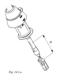
The rigging screw has a stop at the maximum position to which it can be unscrewed. Do not overload this stop by trying to unscrew the rigging screw further. The values given in the table below for adjustment must not be exceeded!
