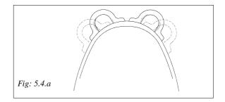
To avoid corrosion between the bronze lead and the aluminium mast, each lead is supplied with a selfadhesive insulator sheet. It is important to fit this between the lead and the mast.
