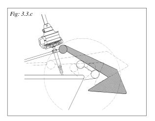
An extension link does not provide the necessary flexibility. It must always have a toggle between it and the boat's forestay attachment.
