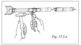
6. Turn the 1000 mm extrusion and the lower bearing assembly upside down. The lower joining sleeve has to be moved 25 mm to allow the parts to be disconnected. This is best done by striking the luff section against something that will not damage it, such as a piece of wood. Strike with the luff section no harder than necessary to move the distance tube and the joining sleeve.
