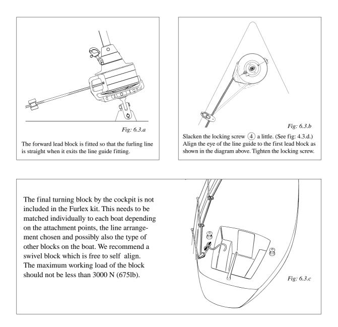
It must be possible to belay the furling line securely. A block with a Cam-cleat works well when securing a reef, but is unreliable if the boat is left unattended. The line should then be secured on a normal cleat for safety reasons. We recommend a single turning block in combination with a cleat.
