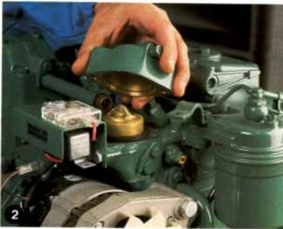
2 Thermostat. The thermostat makes sure that the engine retains the correct working temperature. If your engine is fitted with a temperature gauge you can see if the engine has the correct working temperature.
