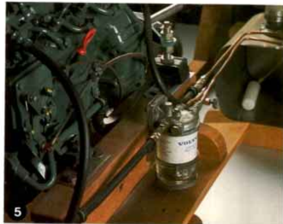
5 Fuel system. Not least important is that you check that the fuel system does not leak. If fuel leaks, then air will also get into the system, and this will cause operational breakdown. For the sake of safety, check the fuel lines now and again.
