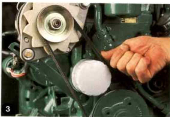
3 Drive belt. Check the drive belt several times a year to make sure that it is tensioned correctly (press the middle of the belt – you should be able to press it down by not more than 5 mm). Also check to make sure it is not cracked or frayed. A worn drive belt will slip and give poor effect to the alternator and, on a fresh-water-cooled engine, to the circulation pump.
