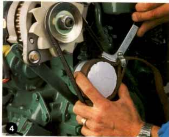
4 Filters. Serviceable oil and fuel filters are a pre-condition in order that the engine shall function properly. These filters are easy to replace, and you should do so after about 100 hours running time or at least once a year.
